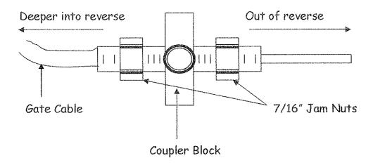
Small adjustments (1/6 of a turn) made with both jam nuts makes a noticeable difference. A smooth shift sequence is therefore attainable first through fourth gears and reverse.
